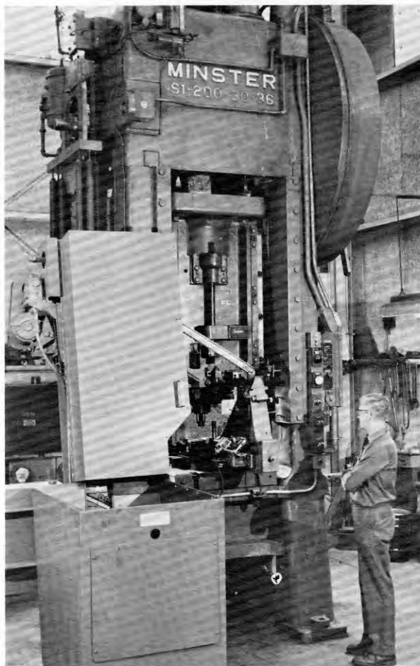
Minster S1-200 press equipped with special parts feeder and tooling developed by Van Epps.
