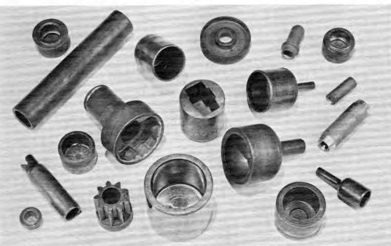
Typical array of cold-formed parts which require little or no machining due to cold flow extrusion process.
