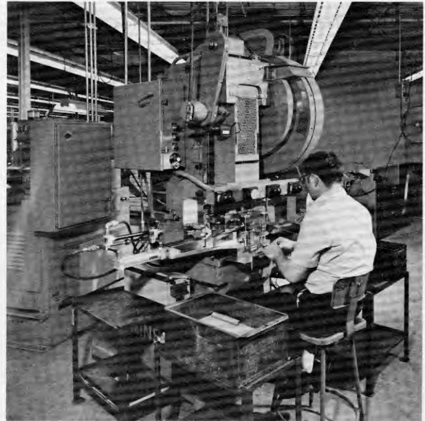
No. 3 O.B.I. is equipped with Urschel designed chute-fed hydraulically-operated automatic sliding parts feeder which eliminates the "hands in the die area" problem, speeds up production and reduces operator fatigue. Each press operator does his own parts inspection.
