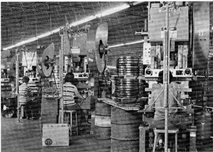
Secondary operations are performed on Minster O.B.I. presses.
