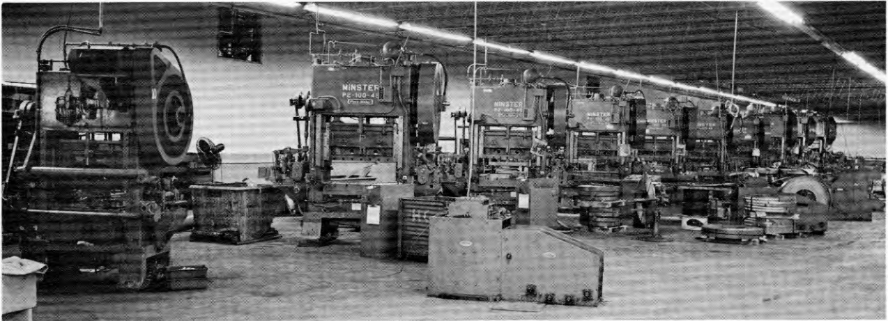
Minster P2 Piece-Maker® high speed automatic production presses ranging in tonnage capacity from 45 to 200 tons give Richmond Tool & Stamping high productivity on a wide variety of parts.
