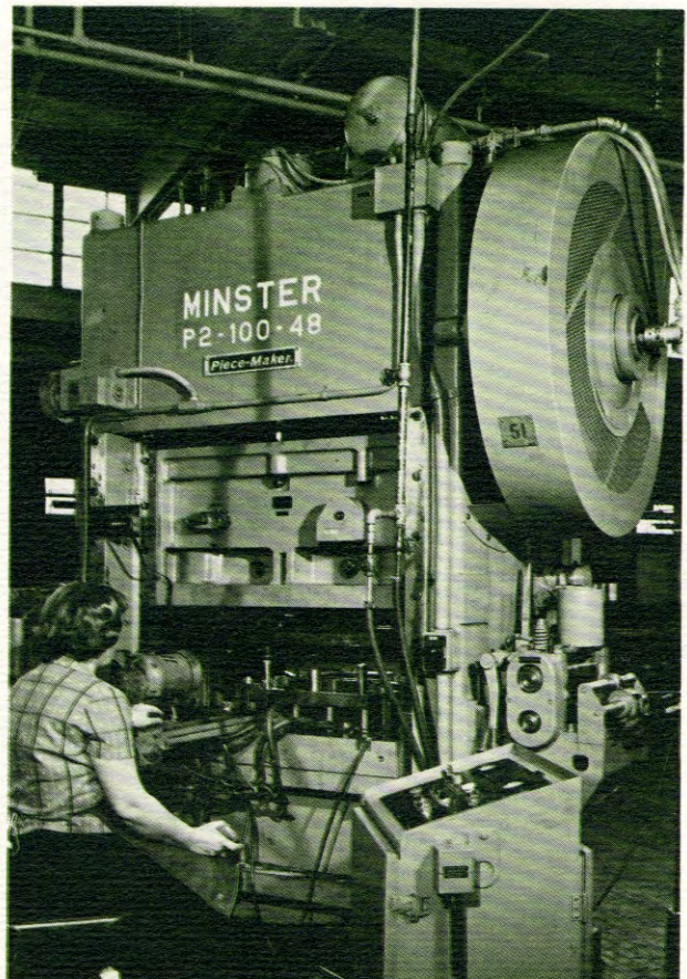
P2 Piece-Maker, 100 tons capacity, with double roll feed and eddy current variable speed drive. Extra shut-height for application versatility. Note conveyor for part removal and easy part inspection.
