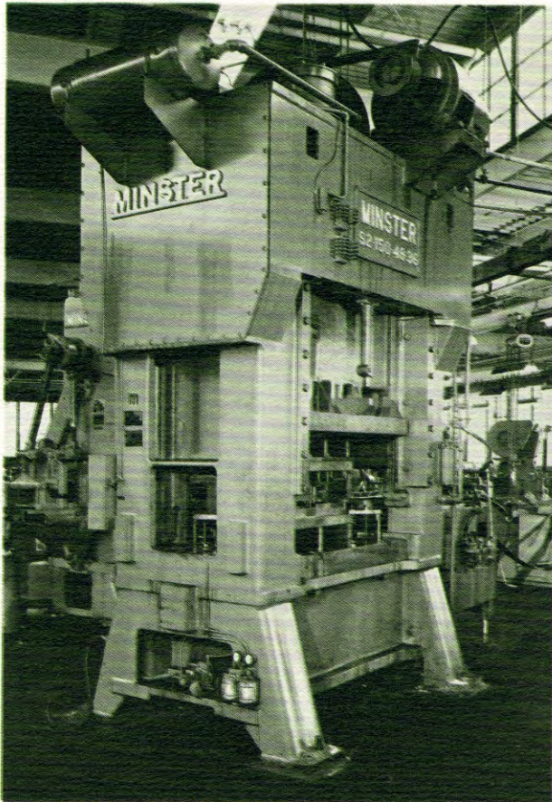
S2 two point straightside press, 150 tons capacity, single-gearred, twin drive, has long stroke and variable speed drive for extra versatility. Equipped with a feeding machine, or can be manually fed. Runs at 40 to 80 spm.
