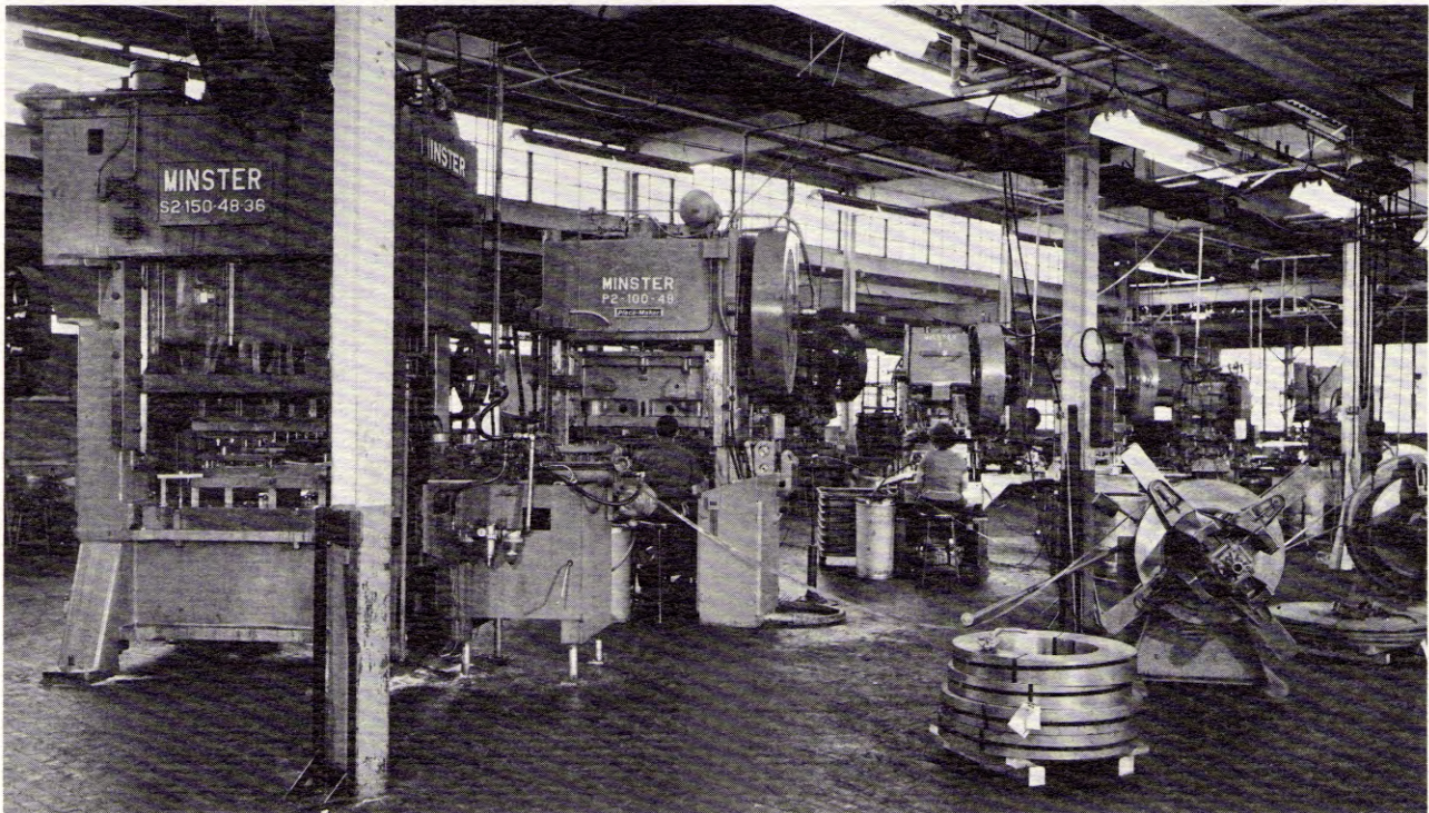
Line of automated Minster presses at Inshield Die & Stamping Co.
