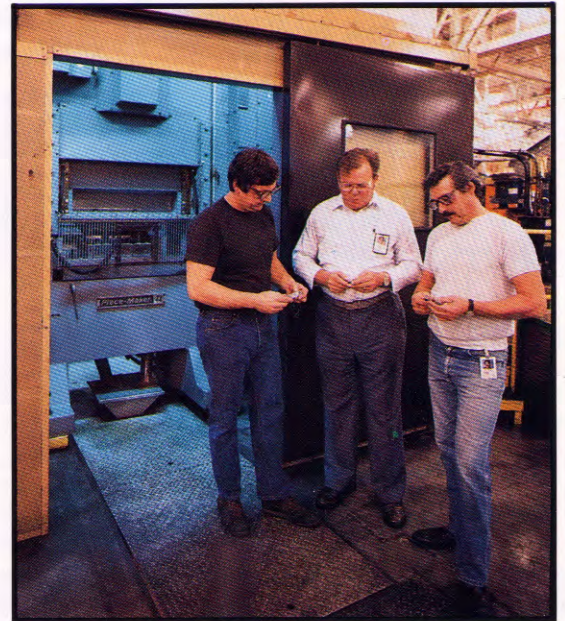
Dennis Scrima, set-up man, John Pasko, Department Foreman, and Roger Bricco, Machine Operator examine the magnet and backpole counterbalance laminations at around the 100 million point. (Looks good for another 20,000,000+!)
