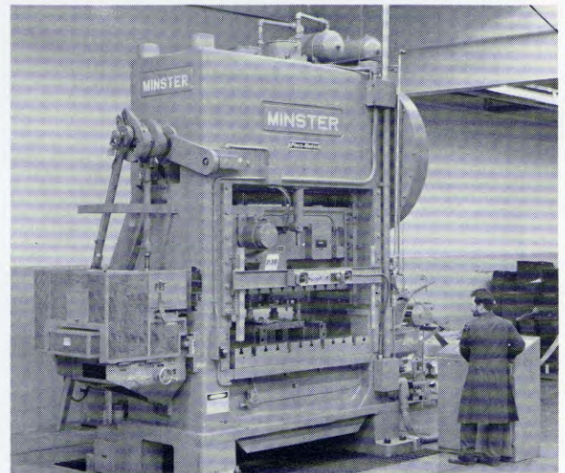
An E2-300 is used for heavy stamping jobs.
