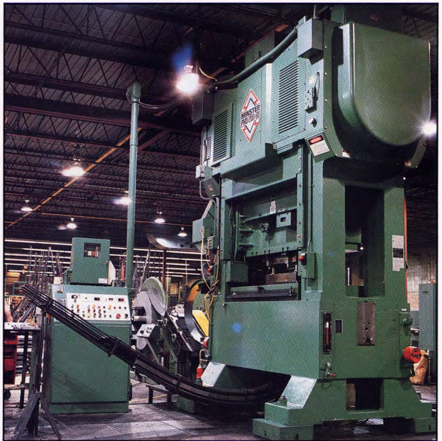
BCL produces loose laminations on this PM3-200 at up to 600 strokes-per-minute. A Minster Cam Feed and "S-Loop" handling system (background) supply material accurately to the press at up to 3700 inches-per-minute.
