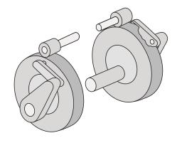
As shown to the left, the ASM option provides reduced slide velocity through the work portion of the stroke and faster slide velocity through the remaining portion of the stroke as compared to a conventional drive running at the same SPM.
