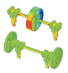
FEA analysis comparing the torsional wind up of a twin drive press to that of a center drive press with the same size shaft shows that when the maximum rated tonnage is applied evenly to each, the vertical deflection of the center drive press is twice that of the twin drive press. The result is a less stiff press and increased punch penetration in snap thru applications.
